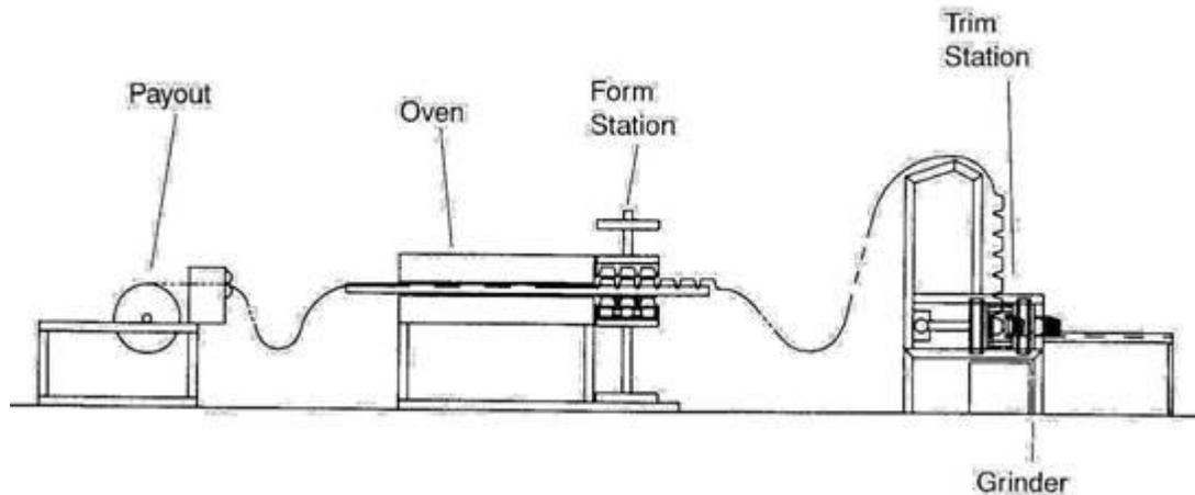
Two-station thermoforming has the most flexibility and can be used to produce parts from general purpose thermoforming grades like PET to engineering grades of plastic and other difficult to form plastics like CPET.
